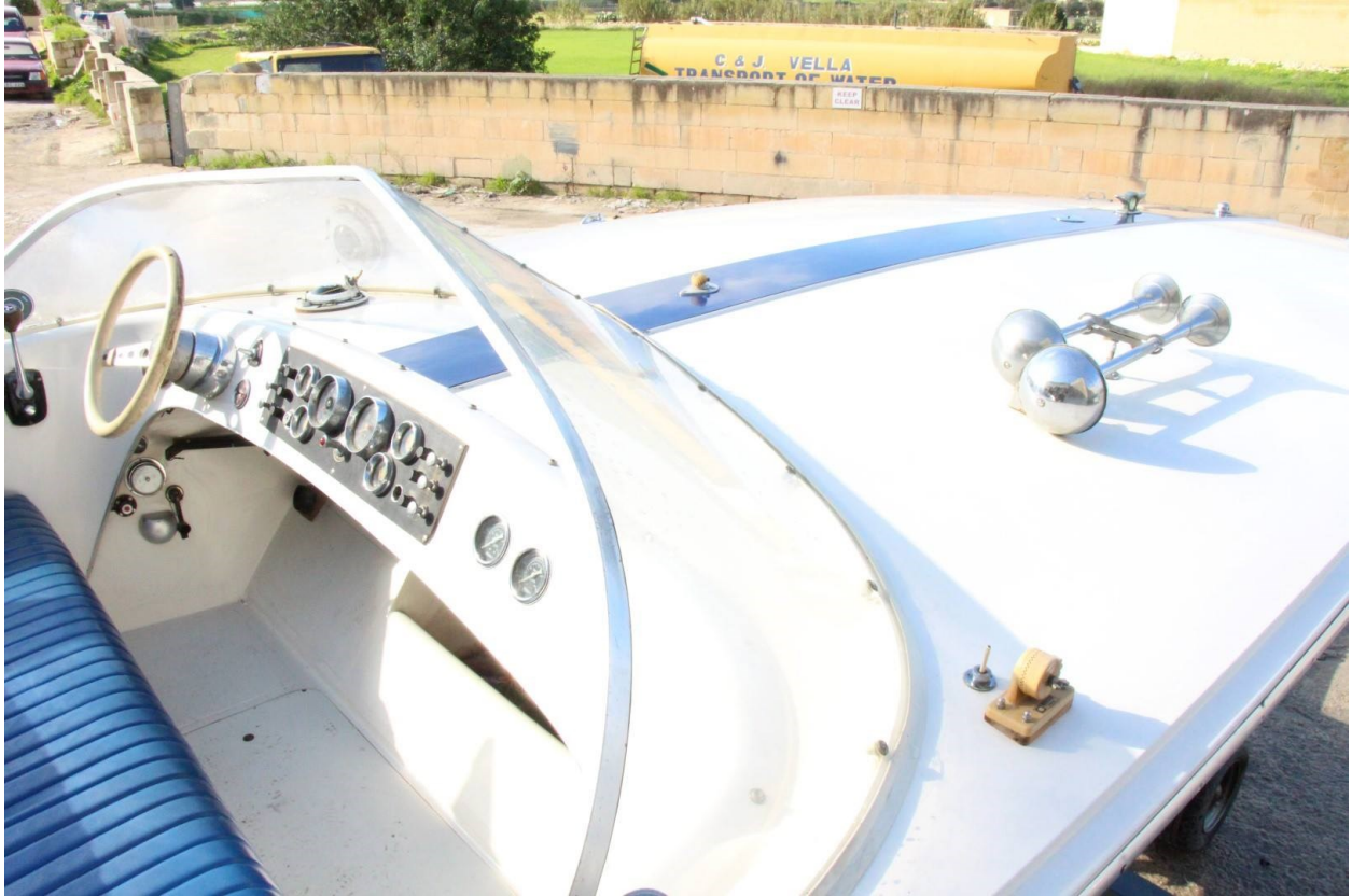
The dash lip on a 1969 boat sweeps down to the floor and the sidewall by the foot well is not diagonal.
