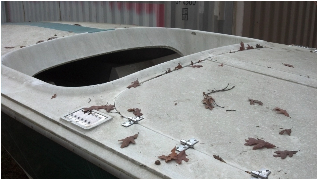
The raised Deck Vents.
