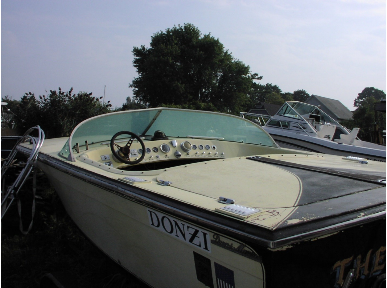
Daytona Turbo boat with Gauges cut directly into the dash.
