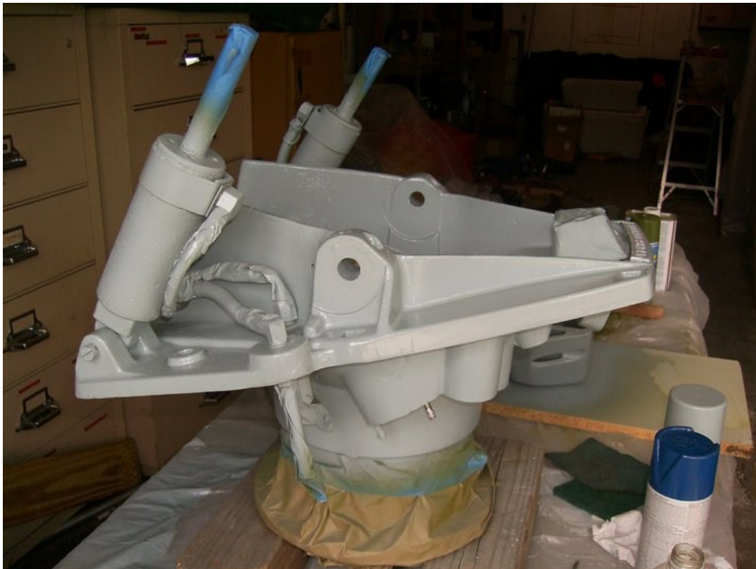
Transom housing was primed in a zinc chromate, and then painted.
