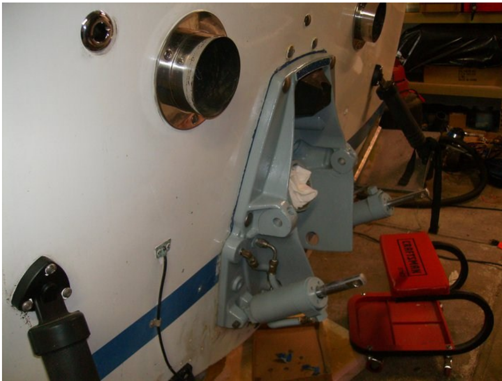
Transom housing re-installed the original blue gel can be seen at the edges.
