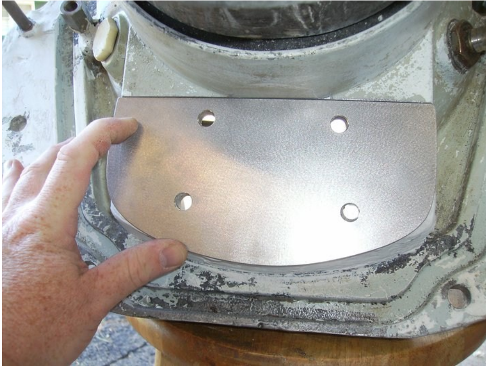
A one off aluminum block off plate was made for the thru hub exhaust.
