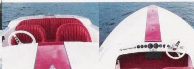
**STANDARD EQUIPMENT — Electrical System:** 12 volt, color coded, fused • **Safety ignition** • **Instruments:** Tachometer, fuel gauge, water temperature gauge, oil pressure gauge, ammeter, engine hour meter, speedometer • **Controls:** Single lever throttle and shift combination •
