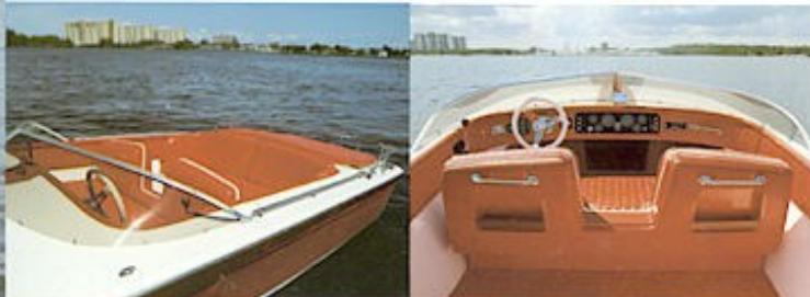
**STANDARD EQUIPMENT** • **Steering:** Teletex mechanical • **Electrical System:** 12 volt, color coded • **Instruments:** Tachometer, speedometer, ammeter, oil pressure, water temperature, electric fuel gauge • **Controls:** Single lever throttle and shift combination • **Battery:** 12 volt, 80 ampere-hour marine • **Fuel System:** 42 gallon aluminum, fully grounded, shutoff, electric gauge, chrome on brass filler and vent
