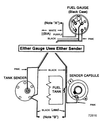
NOTE "A": Connect to "I" (Ignition) Terminal or Accessory Terminal of ignition switch.
